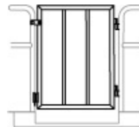
Safety gate option prevents unauthorized access during machine operation.
