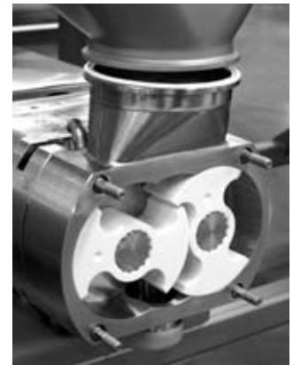
Pump rotor detail shown with cover plate and clamp removed.
